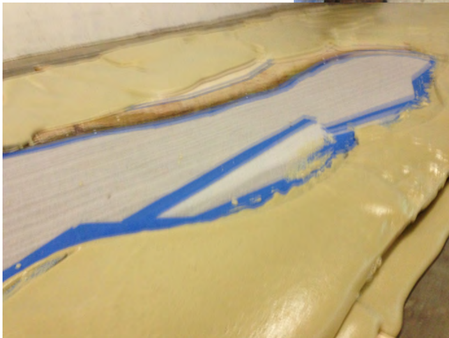
Left: The foam has been poured and is rising to its initial shape. Next steps are to cut the pieces apart so they can be transported, carve the foam and then apply the sand textured surface. Once on site, plants will be added to complete the effect.
